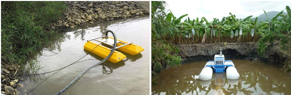
Figure 14: Ideas for designing a floating surface intake for Mardigras
