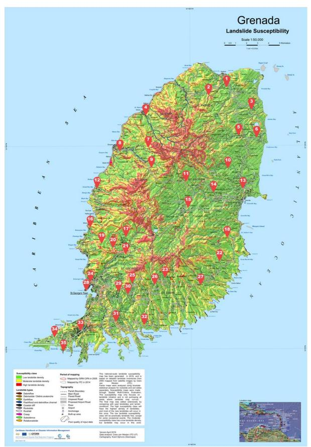
Figure 10. Landslide susceptibility map for Grenada with locations of health centers. (Adapted from: van Westen et al., 2016)
