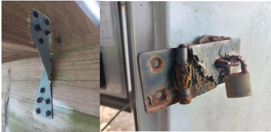
Figure 4.2 - Photos showing corrosion of screws and equipment latch at Blaize
